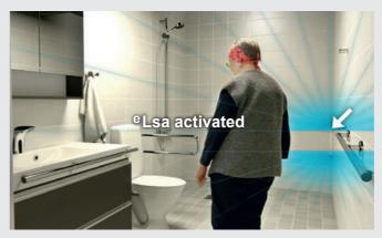
$^{\rm e}\mbox{Lsa}$  is activated when the person enters the room and is detected by the upper motion detector.
