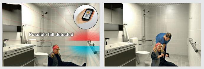
If the person falls, only the lower motion detector detects movement, and <sup>e</sup>Lsa sends an alarm to the preset Smart Phone.
